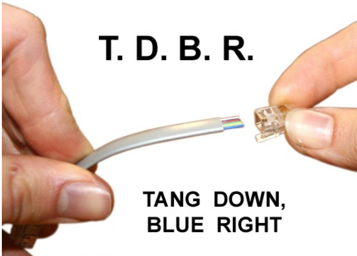
figure 09. Correct RJ Cable Orientation
