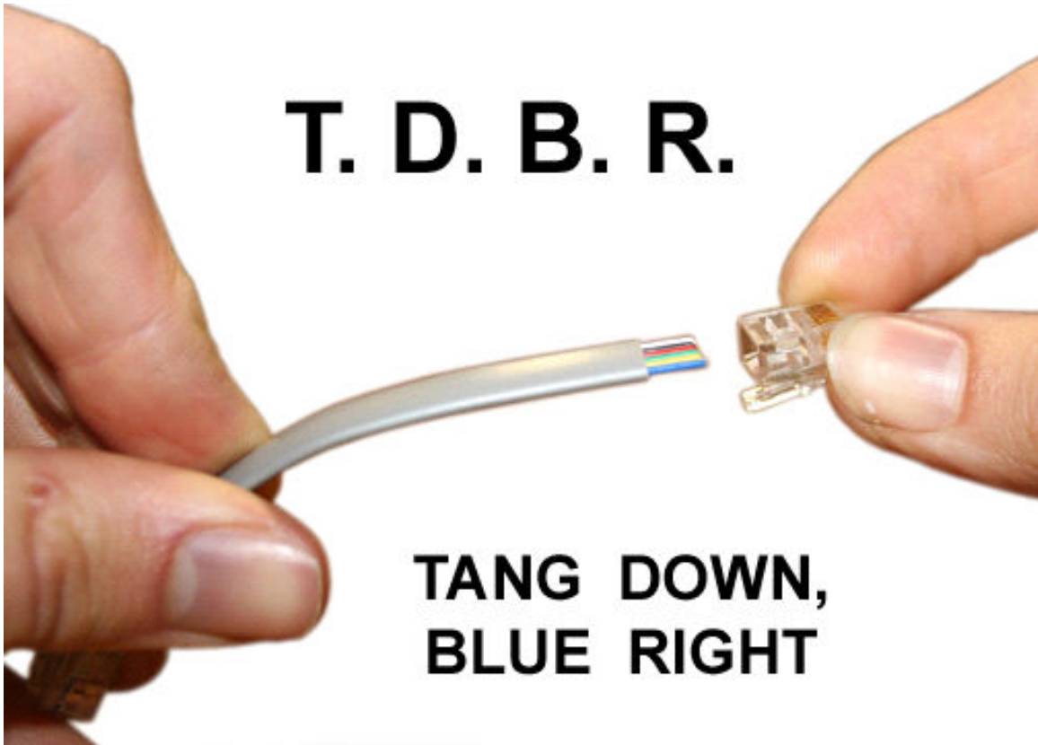
figure 11. Correct RJ Cable Orientation
