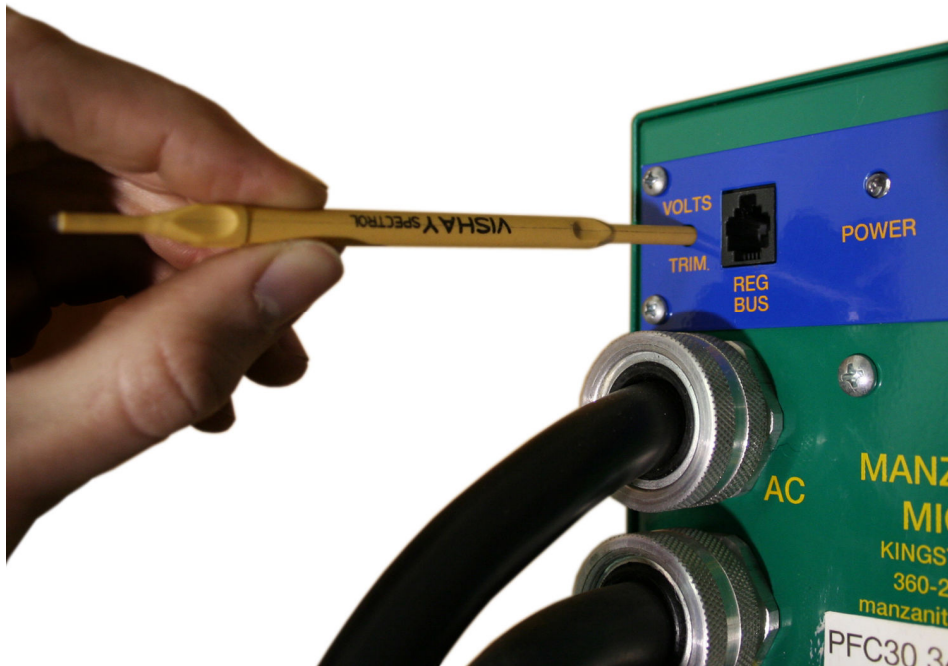
figure 04. VOLTS TRIM Adjustment
