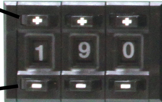
Figure 05 : Optional Digipot Peak Voltage Adjustment
