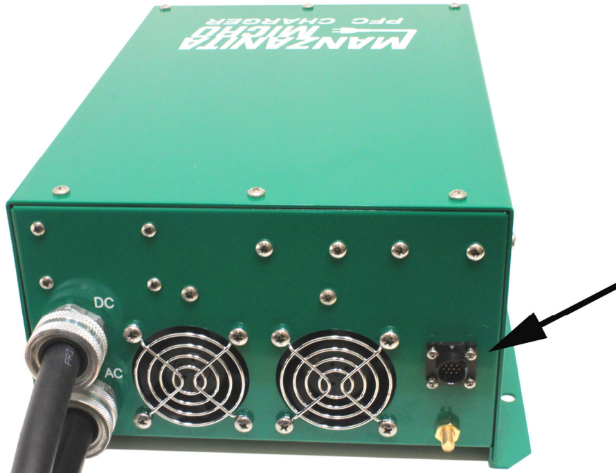
figure 15. Rear Optional Control Port above brass grounding stud on PFC Chargers produced since the end of 2012
